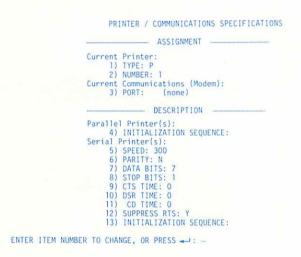
Following are the items on the screen used to describe the characteristics of your printer and Smartmodem. To change an item, enter the item number, PRESS — , and enter the new value. When the change is made, PRESS — to enter the change and PRESS — again to return to the Master Menu.
